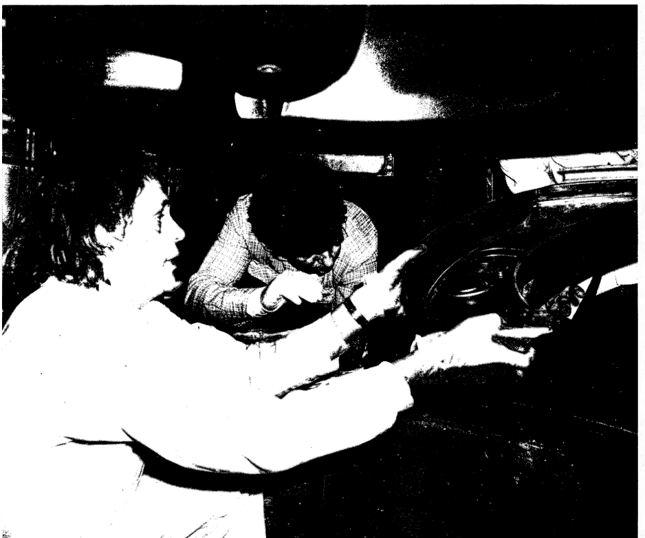
Henry Blosser, Director of the US National Superconducting Cyclotron Laboratory, puts a finishing touch to the machine. He is seen here between the upper and lower pole tips of the magnet installing the 'Dee' electrodes (which in this case are shaped more like giant commas).
